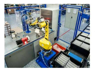
then based on a recommendation by Pierre Rottet from FANUC, and in cooperation with the people at Derap, we opted for these specialised devices." Bürki Electric AG from Steffisburg was responsible for the networking, installation and programming of the PLC controller and the vision components of both systems. Short distances and local companies working hand-in-hand combined to lead this close project collaboration to rapid solutions.
